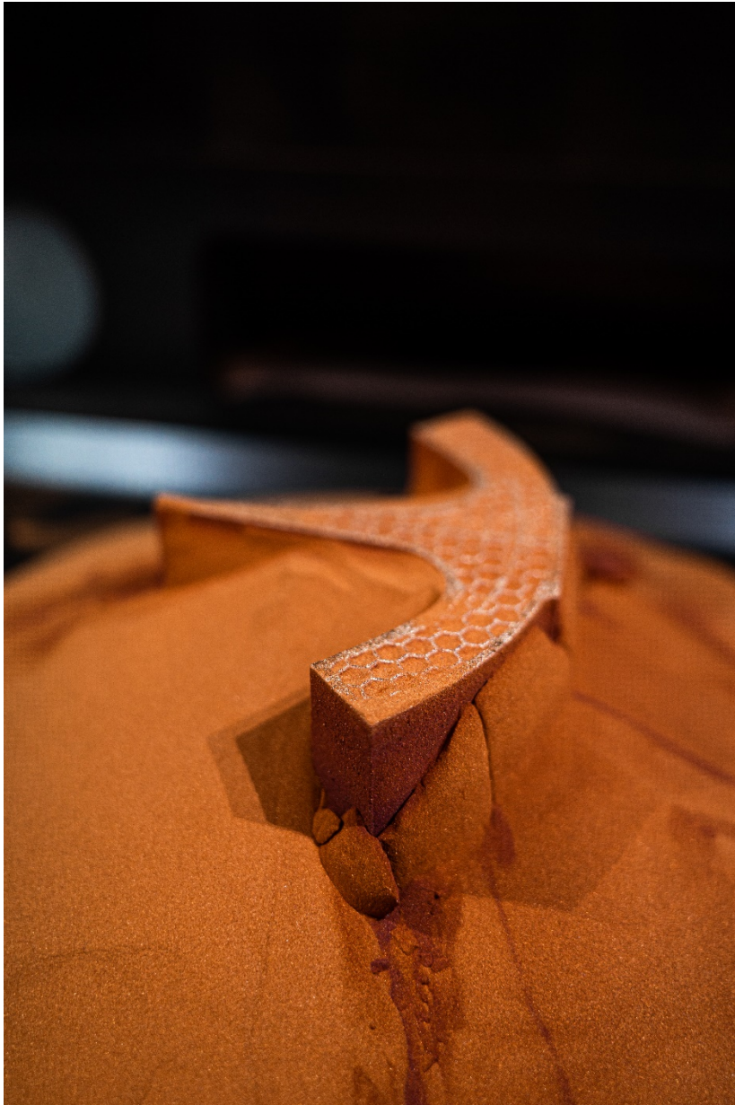
At Fraunhofer IWS, a green laser melts pure copper powder and creates therefrom a quadrupole quarter.
